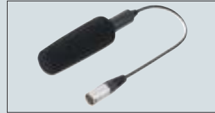
AG-MC200G XLR microphone •Sensitivity: -40 ±3.5 dB (0 dB=1V/Pa, 1KHz) •Maximum input level: 127 dB (1000Hz, Distortion within 1%) •S/N: More than 69 dB
